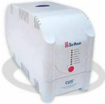
Su-Kams CHIC-800VA, 3-function DC-to-AC inverter with auto AC-to-battery transfer and integrated charging system serves as an extended run standalone power source or a household inverter. This Inverter is designed by using Micro-controller which controls the charging as well as generates PWM at Inverter mode. Supplies up to 560 VA of continuous 220V AC power to one AC outlet from any 12V inverter battery or DC source.
